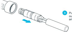
Pull the check valve assembly out of the Tenant Valve Compact and replace for new.
