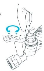
When the desired outlet pressure is reached, push the knob downwards to lock it into place.
